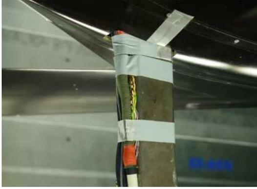
(a) Belly sting mounting at DLR wind tunnel.
