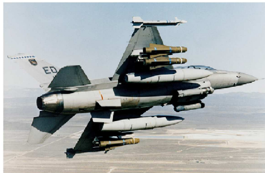
(a) F-16 with ventral fins and LANTRIN pod
