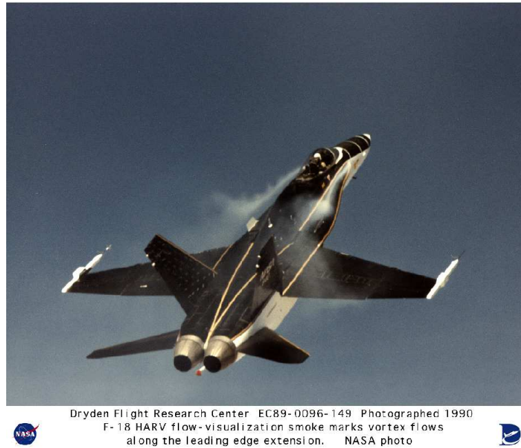
Figure 1.2: Vortex breakdown over the F/A-18 (from ref. [5])
