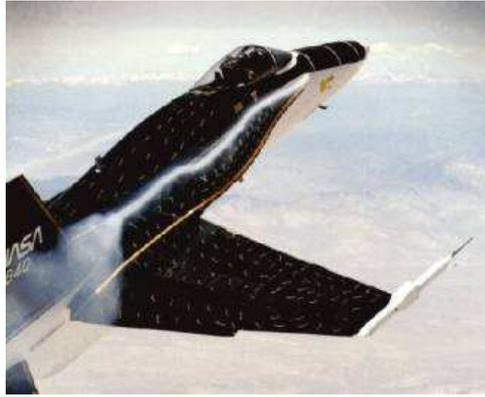
Figure 1.1: NASA F-18 HARV at  $\alpha = 20^\circ$  with smoke visualisation showing vortex created by leading edge extension and vortex breakdown interacting with aircraft tailplane
