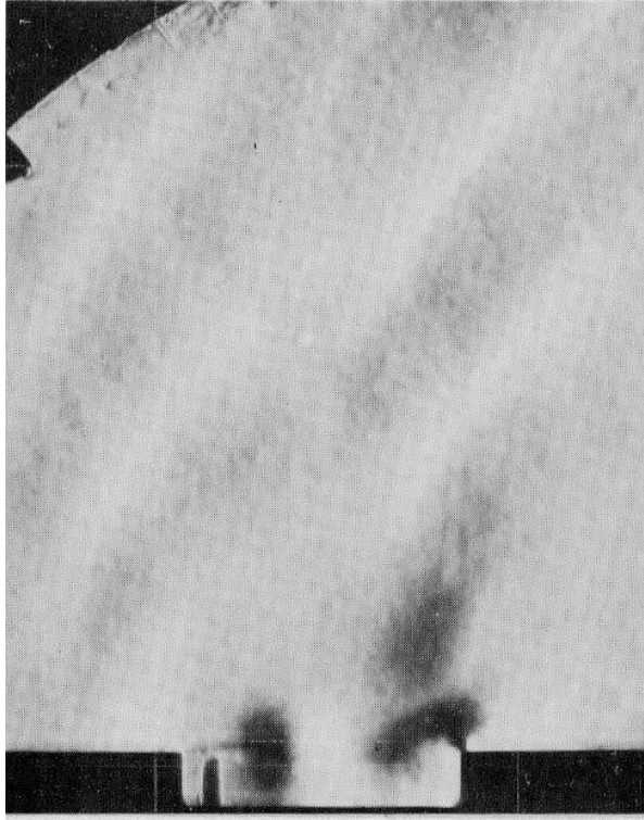
Figure 3.1: Schlieren image by Krisnamurty, L/D=5 Mach 0.804
