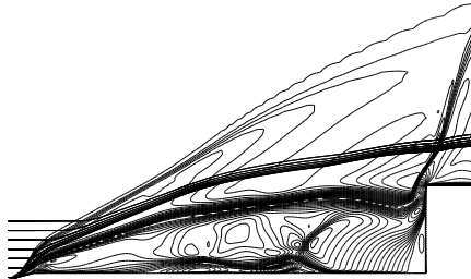
Figure 4.43: The P/O transition occurring at a continuously increasing spike length. Spike speed v_{sp} = 0.004 , freestream Mach number 2.21. Mach number isolines and instantaneous streamlines shown for the frames from Fig. 4.42.
