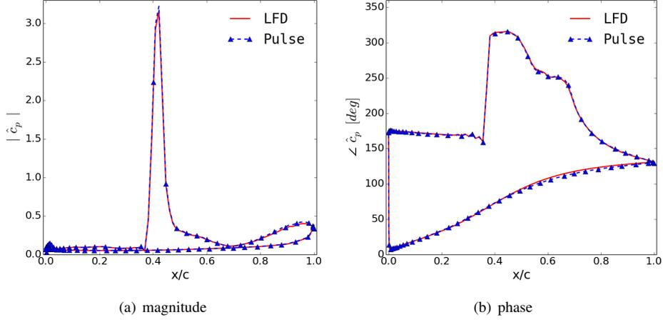
Figure 10: Comparison of complex-valued surface pressures at reduced frequency of 0.5 for wing-body configuration at normalised span position of 0.9
