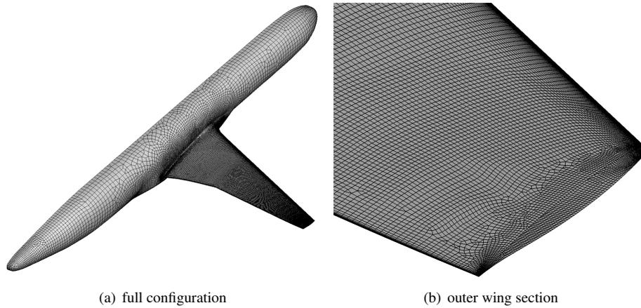
Figure 7: Generic wing-fuselage configuration
