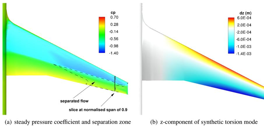
Figure 8: Steady surface pressure and z-component of excitation mode
