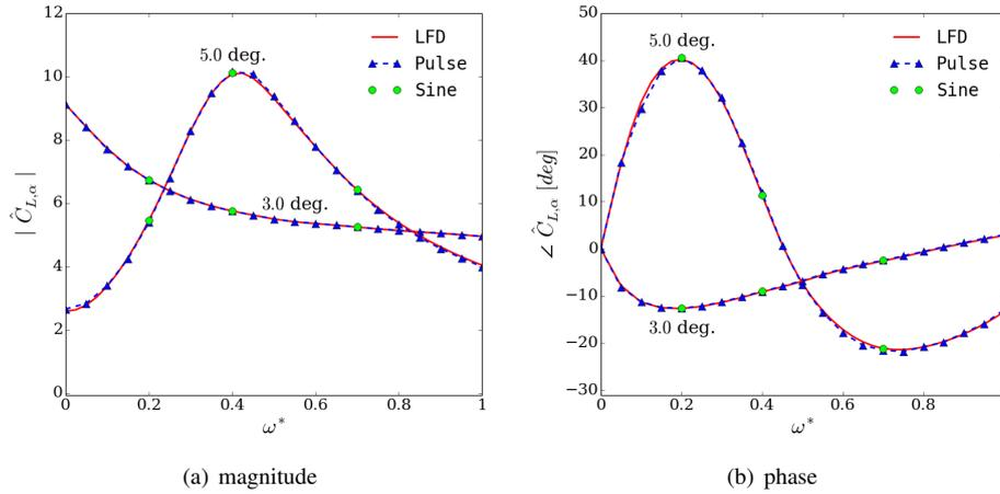
Figure 6: Comparison of frequency responses in lift coefficient for NACA 0010 aerofoil
