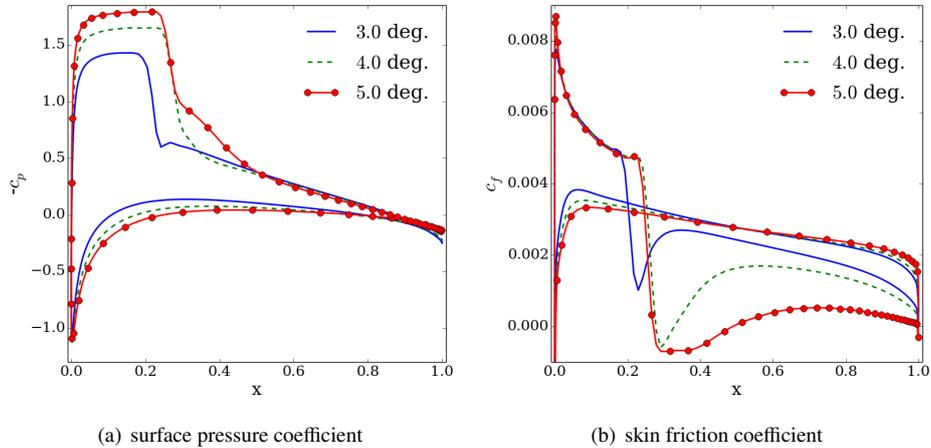
Figure 3: Steady surface pressure and skin friction coefficient for NACA 0010 aerofoil
