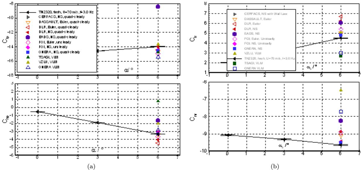
Figure 7. Dynamic Derivatives - a) Unsteady roll motion  $p$ ,  $Ampl. = 4.86^\circ$ ,  $f = 3Hz$ ,  $\beta = 6^\circ$ ,  $V = 70m/s$ ; - b) Unsteady yaw motion  $r$ ,  $Ampl. = 4.32^\circ$ ,  $f = 3Hz$ ,  $\beta = 6^\circ$ ,  $V = 70m/s$ .
