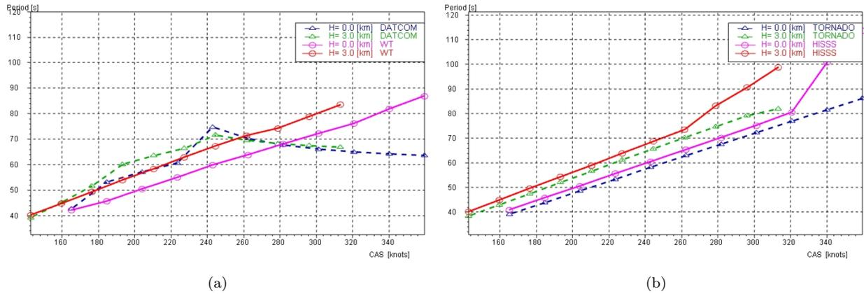
Figure 17. Phugoid period vs calibrated airspeed - results of SDSA for different aero data sets.
