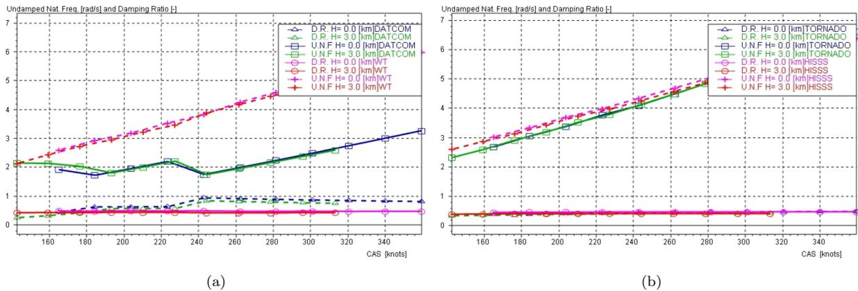
Figure 16. Short Period frequency vs calibrated airspeed - results of SDSA for different aero data sets.
