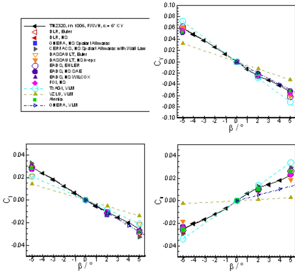
Figure 5. Evolution of the side force, rolling and yawing moment coefficients with sideslip
