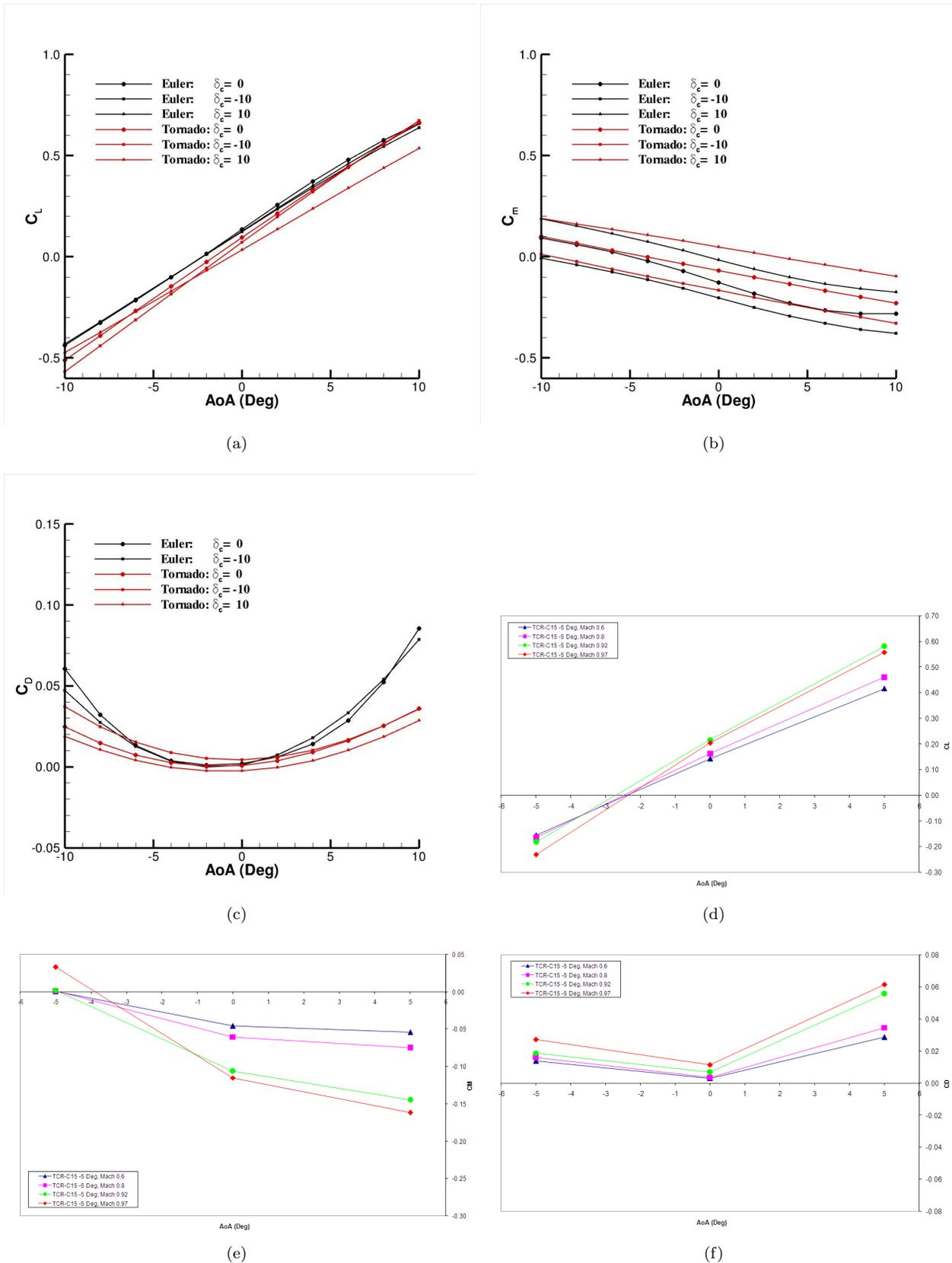
Figure 10. TCR computed aerodynamic coefficients versus  $\alpha$  for various canard deflection angles  $\delta_c$  and: I) low speed  $M_\infty = 0.5$  for a) lift, b) pitch moment, c) drag; II) transonic cruise with canard deflection  $\delta = 0$  for d) lift, e) pitch moment, f) drag.
