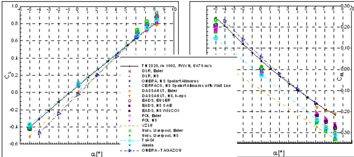
Figure 4. Evolution of lift and pitching moment coefficients with angle of attack
