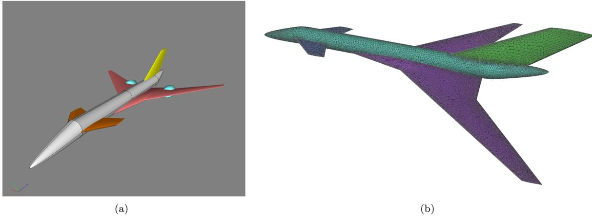
Figure 9. TransCruiser canard configuration a) designed in CEASIOM, and b) sumo surface mesh for Euler
