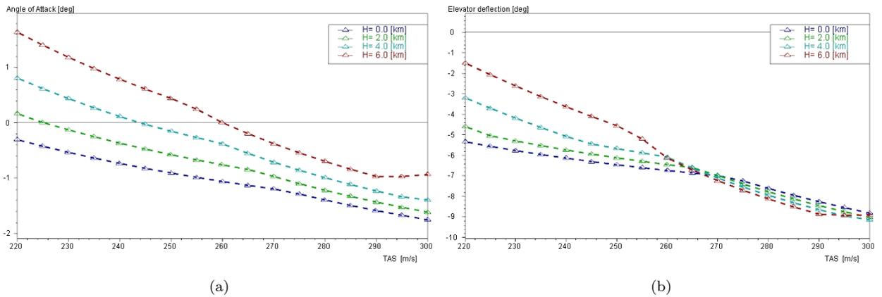
Figure 12. Trim conditions at transonic speed for TCR-C15 : a)angle of attack, and b)canard deflection for various airspeeds and altitudes.
