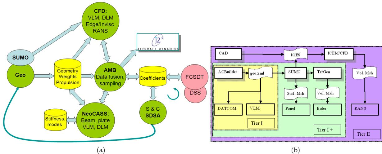
Figure 1. CEASIOM Software - a) Core modules **Geo-sumo**, **AMB-CFD**, **NeoCASS** and **S&C** in the CEASIOM software; - b) **Geo-sumo** software chain: from **Geo** to **CFD** grids.
