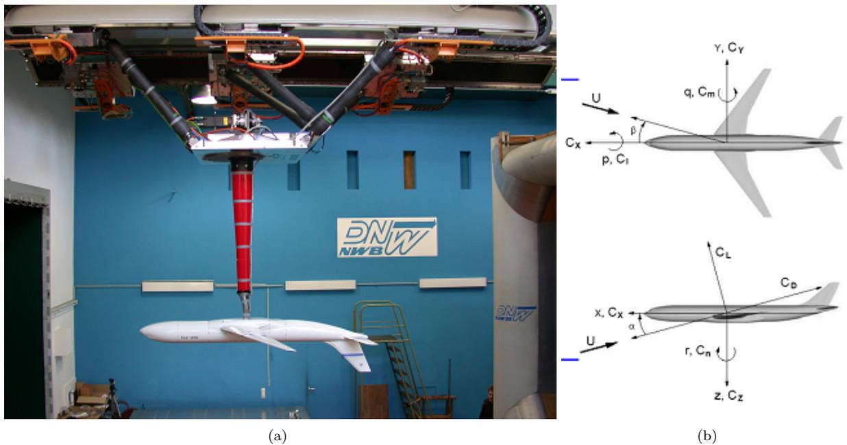
Figure 3. Windtunnel measurements of F12. a) DLR-F12 model on the MPM, b) Axis-system for force coefficients
