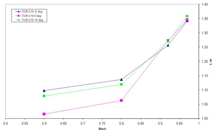
Figure 13. Aero center shifts aft with increasing Mach number
