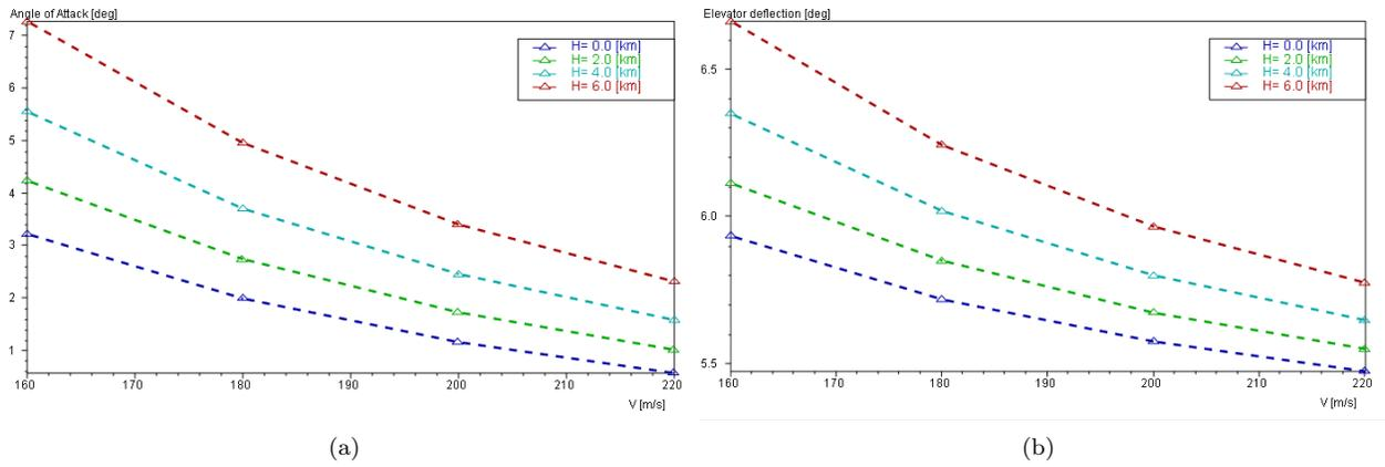
Figure 11. Trim conditions at low speed for TCR-C15 : a)angle of attack, and b)canard deflection for various airspeeds and altitudes.
