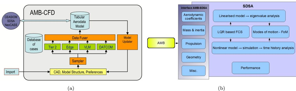
Figure 2. AMB-CFD and S&C Modules: a) Architecture of the Aerodynamic Dataset Generator AMB-CFD; b) SDSA structure and functionality.
