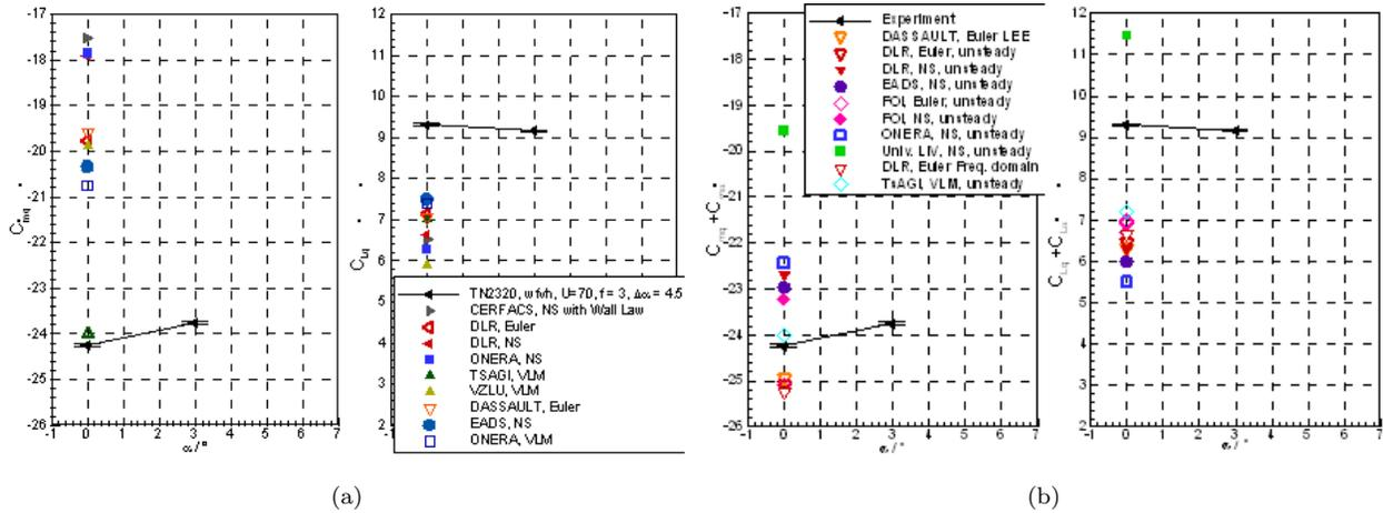
Figure 6. Pitch Motion  $q$  - a) Steady Dynamic Derivatives obtained with Quasi-Steady Tools,  $Ampl. = 4.52^\circ$ ,  $f = 3Hz$ ,  $\alpha = 0^\circ$ ,  $V = 70m/s$ ; - b) Unsteady Dynamic Derivatives obtained with Unsteady and Frequency Domain Tools,  $Ampl. = 4.52^\circ$ ,  $f = 3Hz$ ,  $\alpha = 0^\circ$ ,  $V = 70m/s$ .
