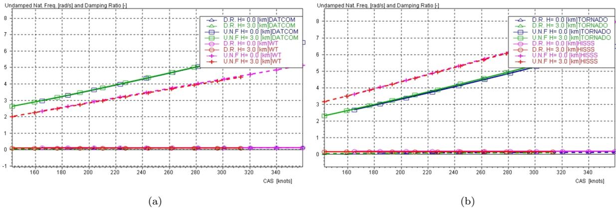
Figure 18. Dutch Roll frequency vs calibrated airspeed - results of SDSA for different aero data sets.
