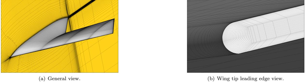
**Figure 7. RLE configuration structured grid.**
