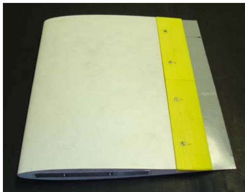
Figure 2. (a) NACA0012 airfoil model with a Mylar SETE, (b) Baseline model, removable parts, and aluminum SETE and Mylar SETE.
