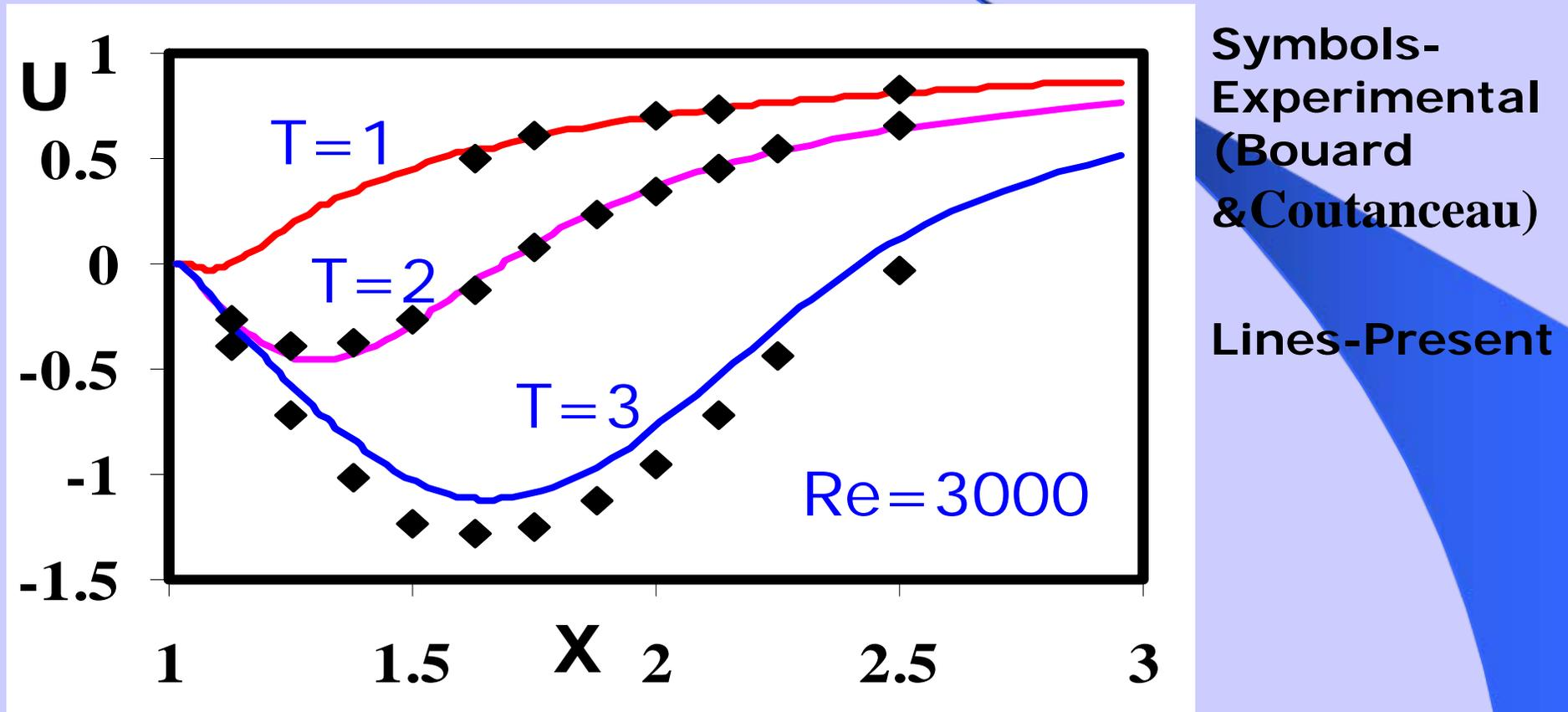
Fig.11 Flow at Early stage at  $Re = 3000$  (Radial Velocity Distribution along Cut Line)
