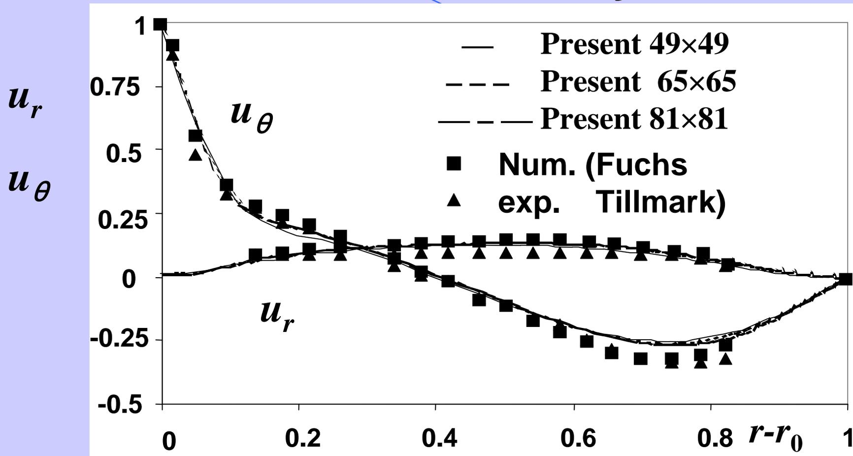
Fig.4 Radial and azimuthal velocity profile along the line of  $\theta=0^\circ$  with  $Re=350$
