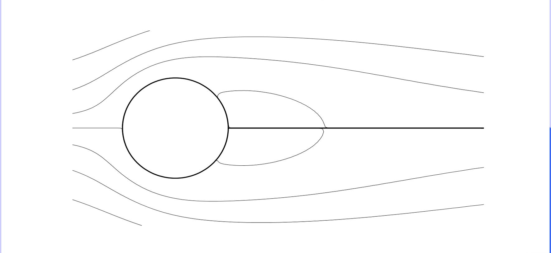
Fig.8 Flow at  $Re = 20$  (streamlines)
