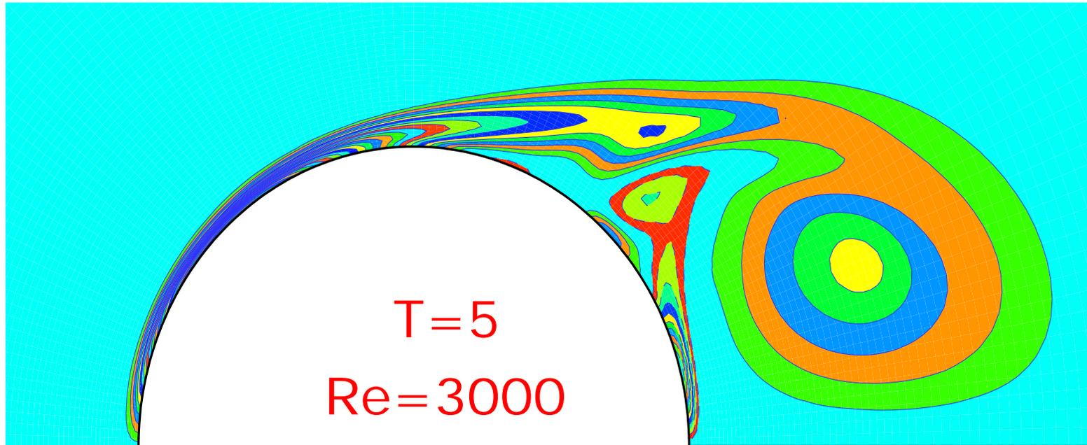
Fig.10 Flow at Early stage at  $Re = 3000$
