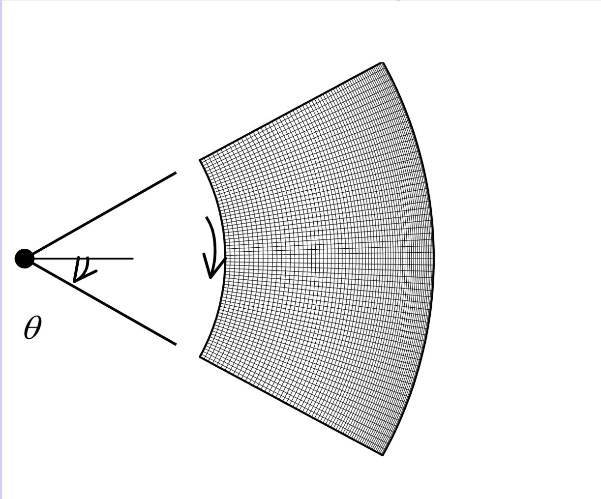
**Fig. 3 Sketch of polar cavity and mesh**
