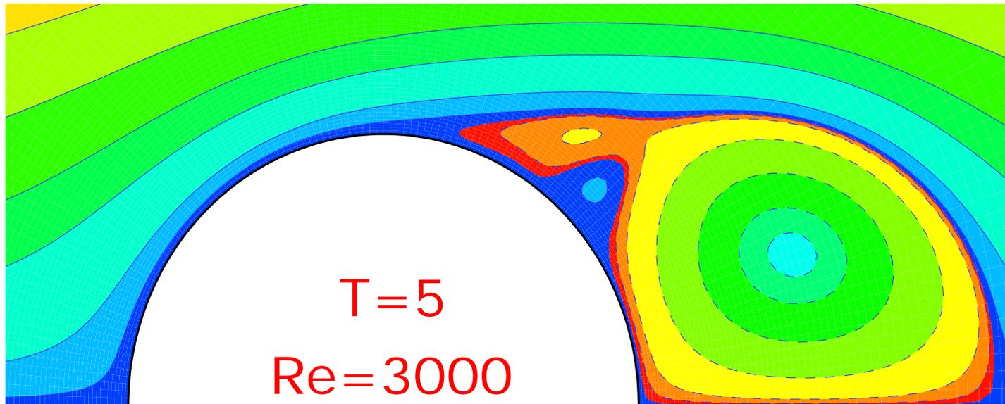
Fig. 9 Flow at Early stage at  $Re = 3000$
