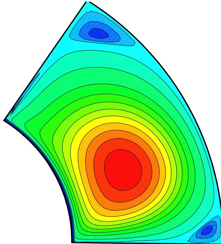
**Fig. 5 Streamlines in Polar Cavity for  $Re=350$**
